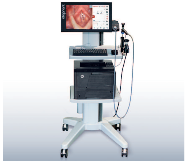
The picture shows the stroboscope on a trolley with printer and storage quivers for endoscopes
